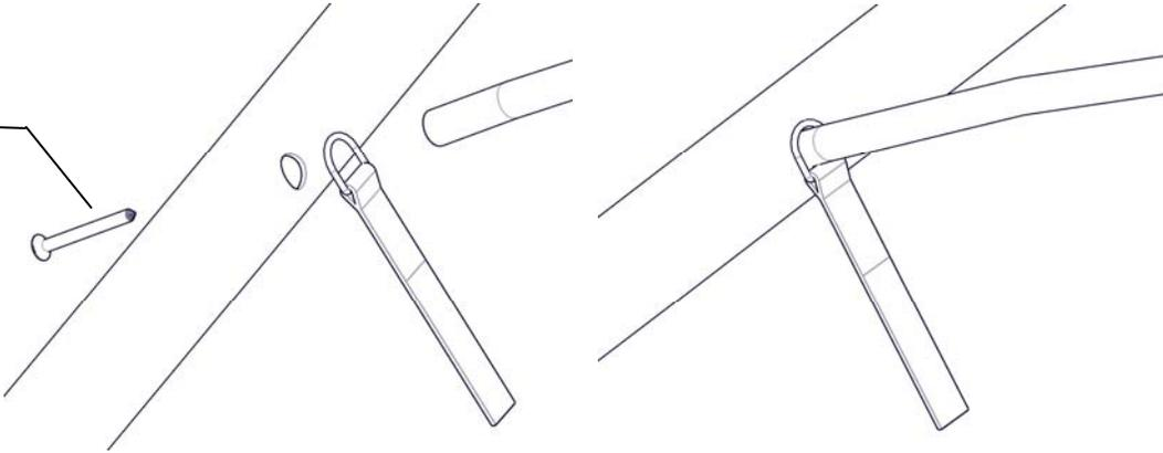
Secure Rafters & D-Ring Velcro Straps. Fasten the rafter and install the High Wind Strap. Sink screws into tubes until head is flush with surface.
