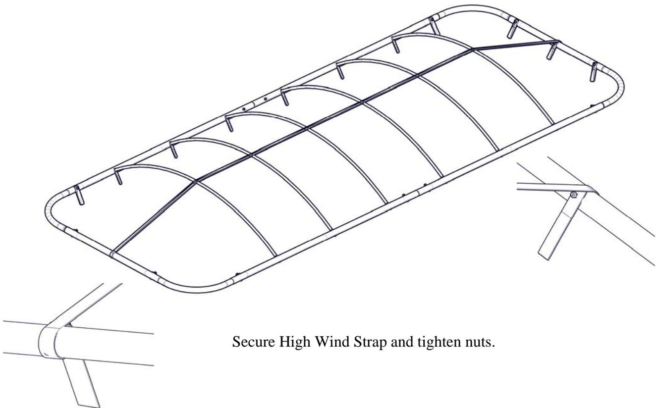
Secure High Wind Strap and tighten nuts.
