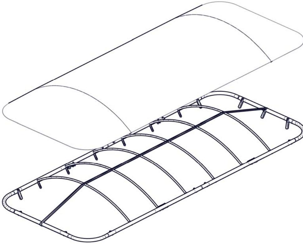
Lay fabric over frame, then pull the three pockets over the corners of the frame while leaving the pull strap pocket for last. Pull 4th corner over with pull strap.
