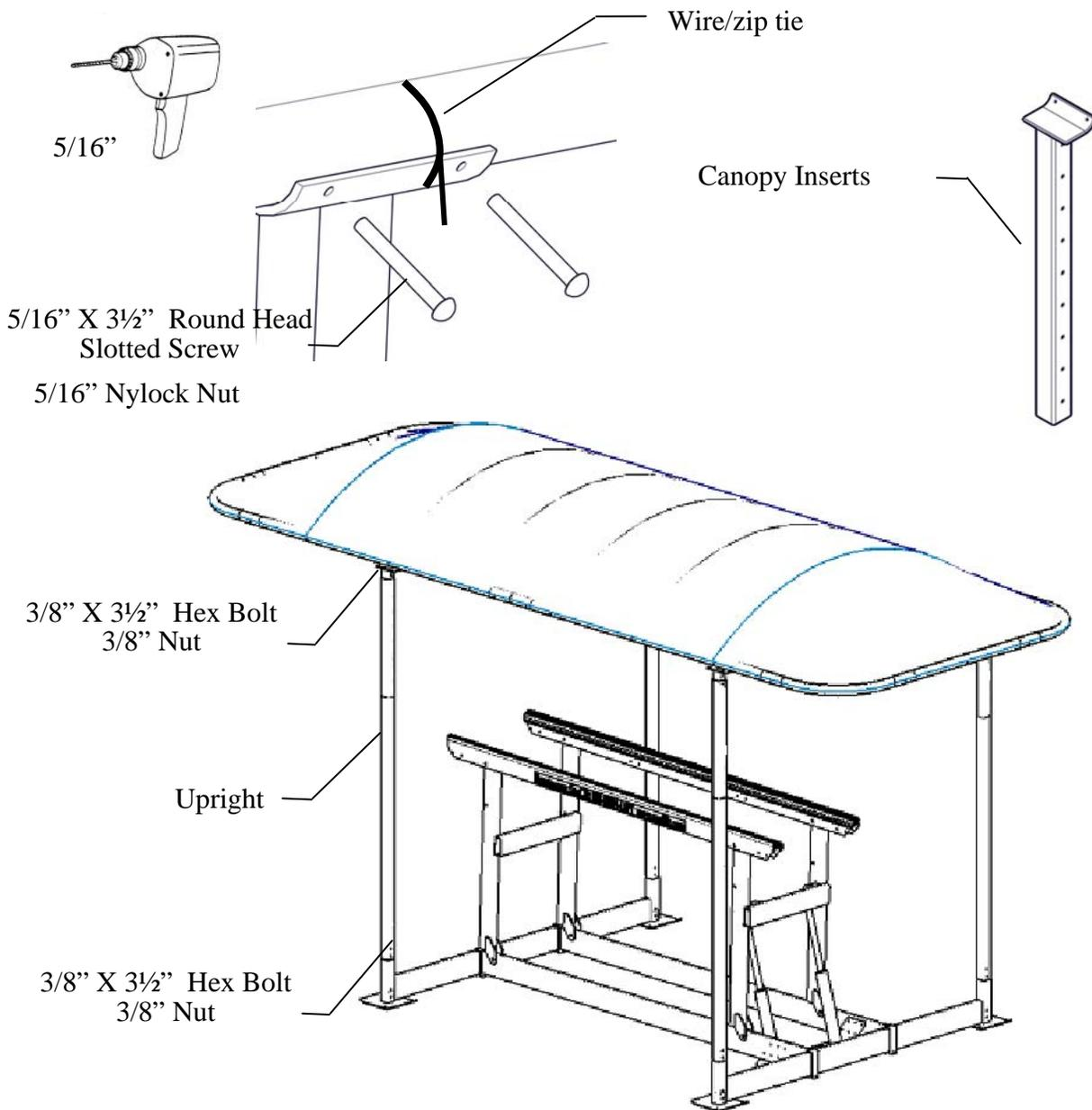
Set Canopy Inserts into the uprights and loosely fasten the fasteners.
