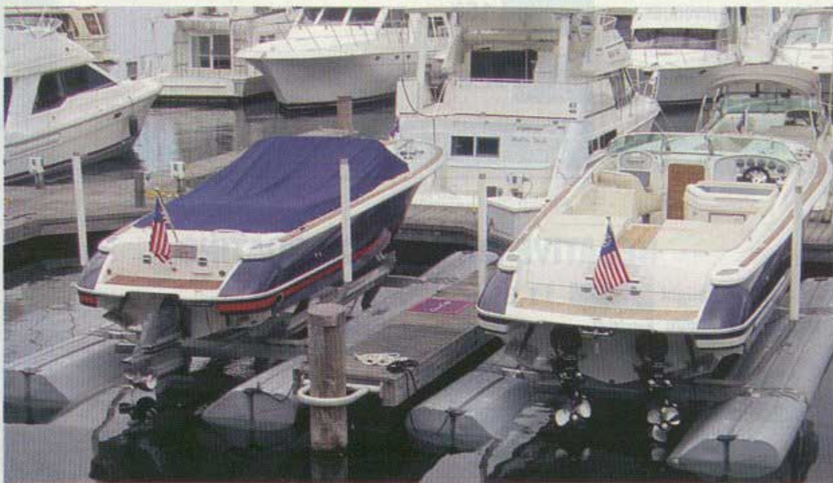
Sunstream Floatlifts are made of an aluminum frame, are hydraulically powered, and can lower a boat into the water in less than 30 seconds.
